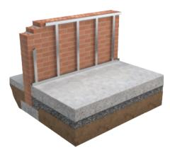
**4.** Lift the SR/TB-MF into position using wedges on the floor. Insulation should be cut back to accommodate an adjoining panel at external corners. Joints should be tightly butted.
