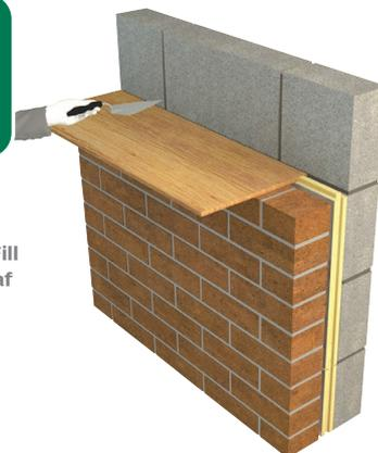
Figure 2 - Use of Eco-Cavity Full Fill when installing the inner wall leaf
