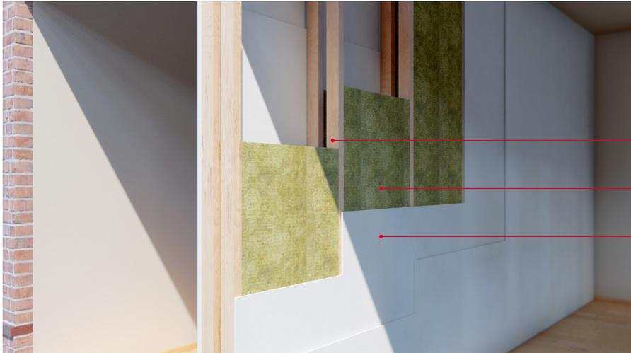
Twin timber frame with 50mm gap between
