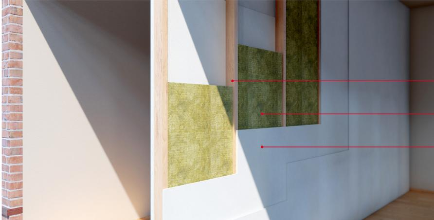
38 x 75mm timber studs at 600mm
