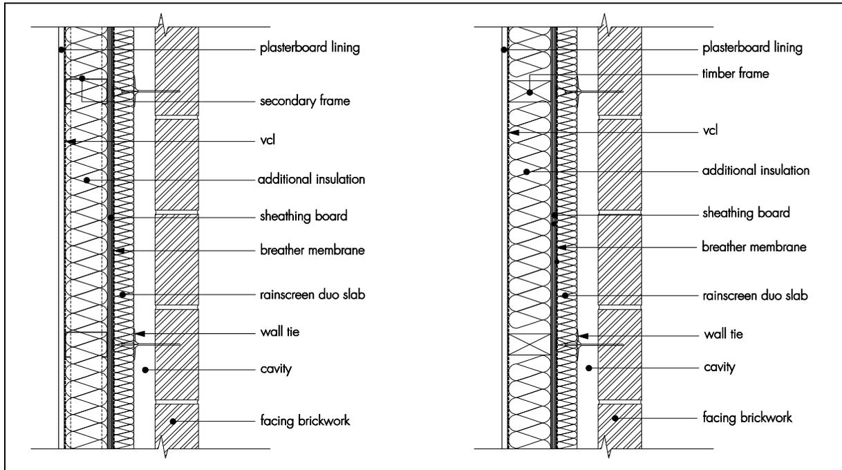
15.5 The insulation should be installed to coincide with the steel/timber frame, with retaining discs used in conjunction with the wall ties at no more than 600 mm horizontally and 450 mm vertically.
