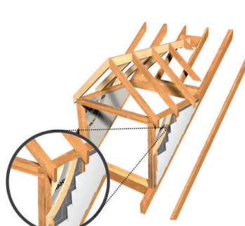
Timber frame wall with weatherboards
